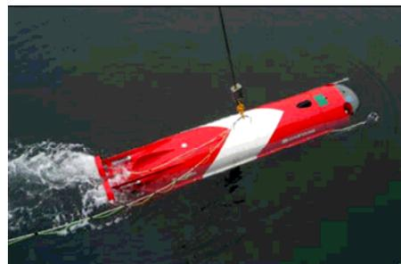
AUV for Dual-Purpose Usage (2003, MOERI)
