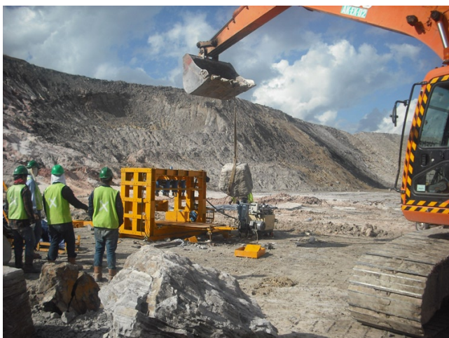
Fig. 1 A process to perform "direct shear test" for big rock specimen at Adaro Coal Mine, South Kalimantan.
