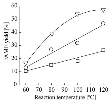
**Fig. 4.** Effects of catalyst concentration on FAME yield: Reaction temperature □, 60 °C; ○, 80 °C; △, 100 °C; ▽, 120 °C; Molar ratio of methanol to oil = 6:1; Reaction time = 30 min.
