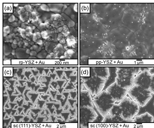
**Fig. 1.** Crystallization of 5 nm-Au colloids on (a) rp-, (b) pp- and (c, d) sc-YSZ ((111) and (100), respectively) plates, after annealing at 1000°C for 2 h.
