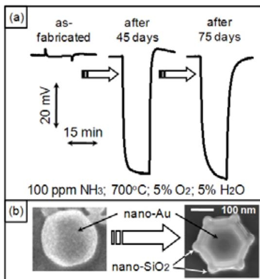
**Fig. 4.** (a) Response transients to 100 ppm  $\text{NH}_3$  at 700°C under the wet condition for the sensor based on pp-YSZ treated with 5 nm-Au; (b) change of the shape of spherical Au particles to hexagonal-like Au-SiO<sub>2</sub> composite.
