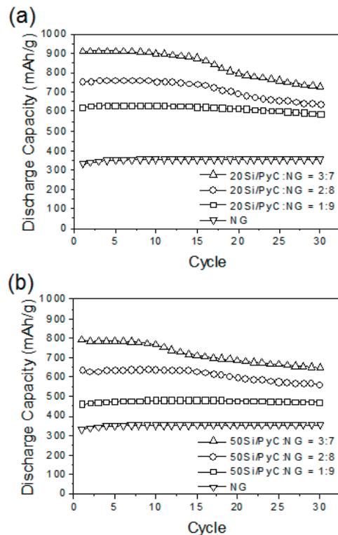
**Fig. 5** Cycle-ability of Si/PyC mixed natural graphite hybridized materials at the current density of 30 mA/g, (a) 20Si/PyC mixed natural graphite hybridized materials, (b) 50Si/PyC mixed natural graphite hybridized materials.
